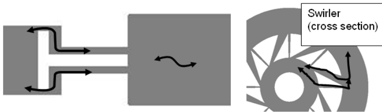
(a) Acoustic wave propagation through the swirler.
